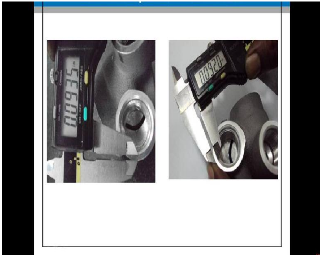
Fig.12 Valve plate with improved valve thickness
